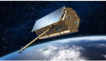
The German radar satellite TerraSAR-X will orbit the Earth in a polar orbit at a height of 514 kilometres; using the mission's newly designed active antenna, it will gather high-quality X-band radar data from the entire planet. TerraSAR-X will operate independent of weather conditions, cloud coverage or lighting and will supply radar data at a resolution of up to 1 metre.
