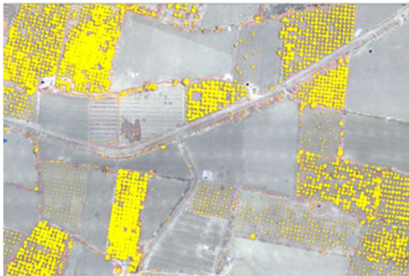
Citrus orchards extracted using RF classifier
