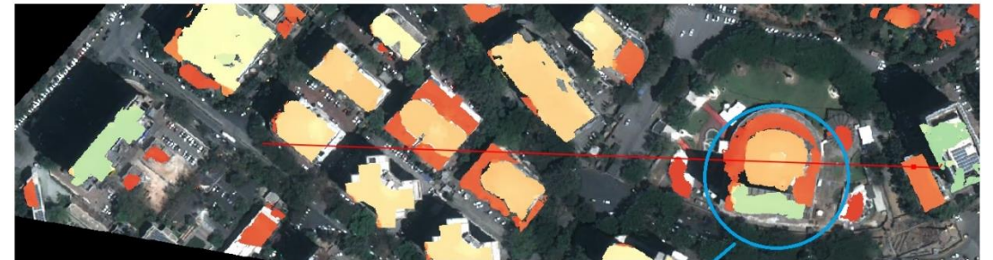
Buildings Extracted DSM overlayed on top of orthoimage(RGB)
