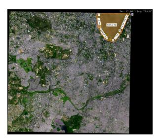
**Distance Measurement Tool:** Distance/Length of any feature on the Image can be measured by the distance measurement Tool as shown below:
