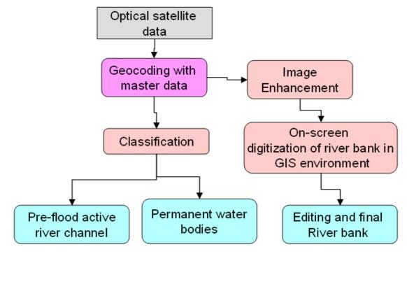
Figure.3. Methodology for Pre-flood data preparation
