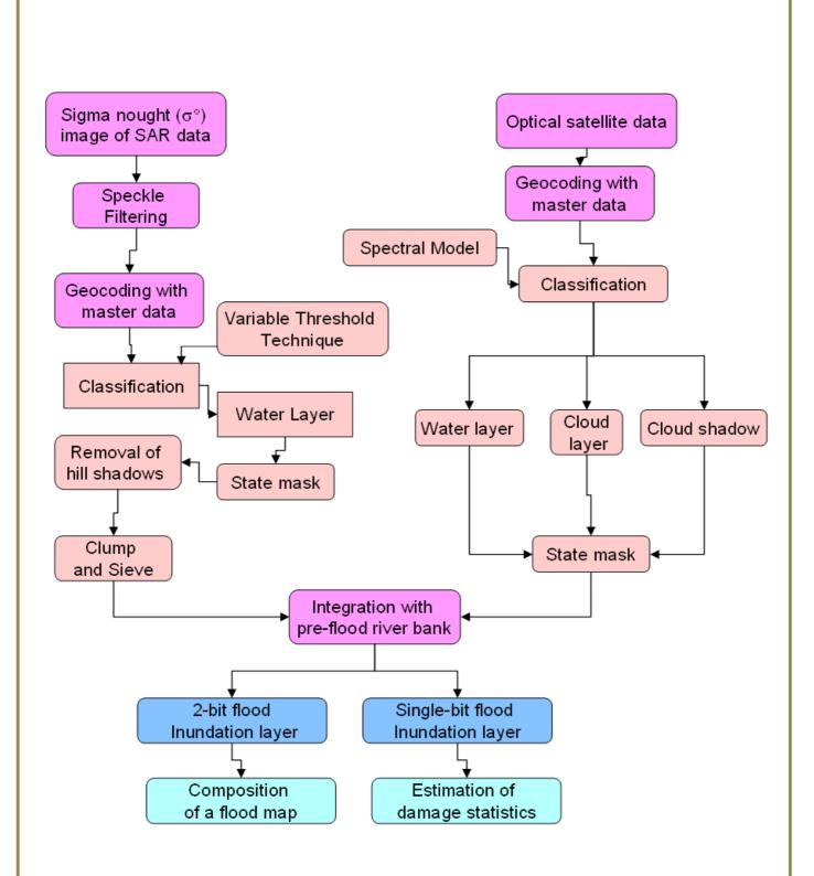
Figure.4. Methodology for flood mapping and monitoring
